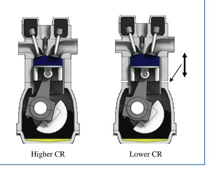
The desired compression ratio can be achieved by vertically lifting the engine head and bore together, resulting in increased clearance volume. The variable compression ratio is achieved without change in combustion chamber geometry. Operate on both SI and CI mode without changing the engine head.
