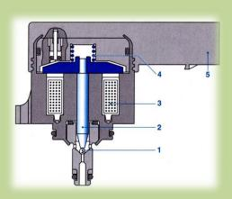
mechanical pressure damper; smoothing the high frequency pressure pulses emanating from the radial piston pump when less than three pistons are activated.
