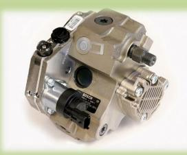
pistons of the pump are able to be shut down. This is achieved by using a solenoid to hold the intake valve of that piston open. However, when a piston is deactivated, the fuel delivery pressure fluctuates to a greater extent than when all three pistons are in operation.
