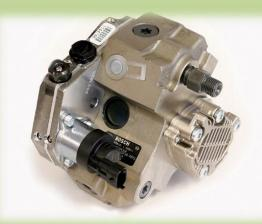
pistons of the pump are able to be shut down. This is achieved by using a solenoid to hold the intake valve of that piston open. However, when a piston is deactivated, the fuel delivery pressure fluctuates to a greater extent than when all three pistons are in operation.
